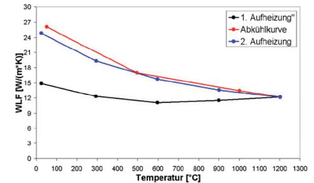
**Fig. 1:** The thermal conductivity of a castable containing SiC during the first heating, the following cooling and the second heating. Measured by hotwire-parallel-wire.
