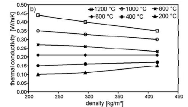
**Fig. 2:** The thermal conductivities of high temperature insulation wool depending on the bulk density (compression) and the temperature. Measured by the method of Monotonic Heating.
