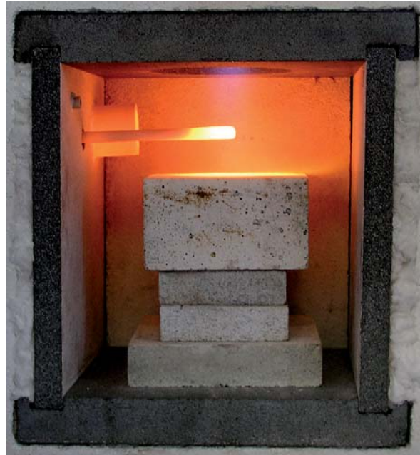
Fig. 1: Blast wear test at elevated temperature.
